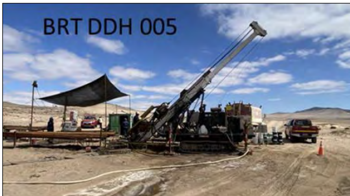
Figure 10-5. Diamond drill hole rig set up at hole BRT-DDH-005 (Fitzroy, 2024).
