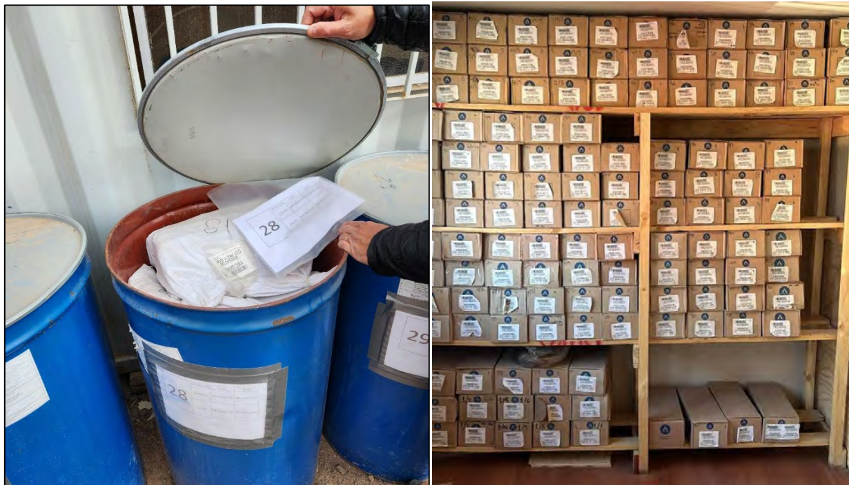
Figure 11-2. Rejects (left) and Pulps (right) from the 2023-2024 diamond drilling program are stored in labelled and weatherproof barrels at the rented warehouse, south of Copiapó (Caracle Creek, 2024).
