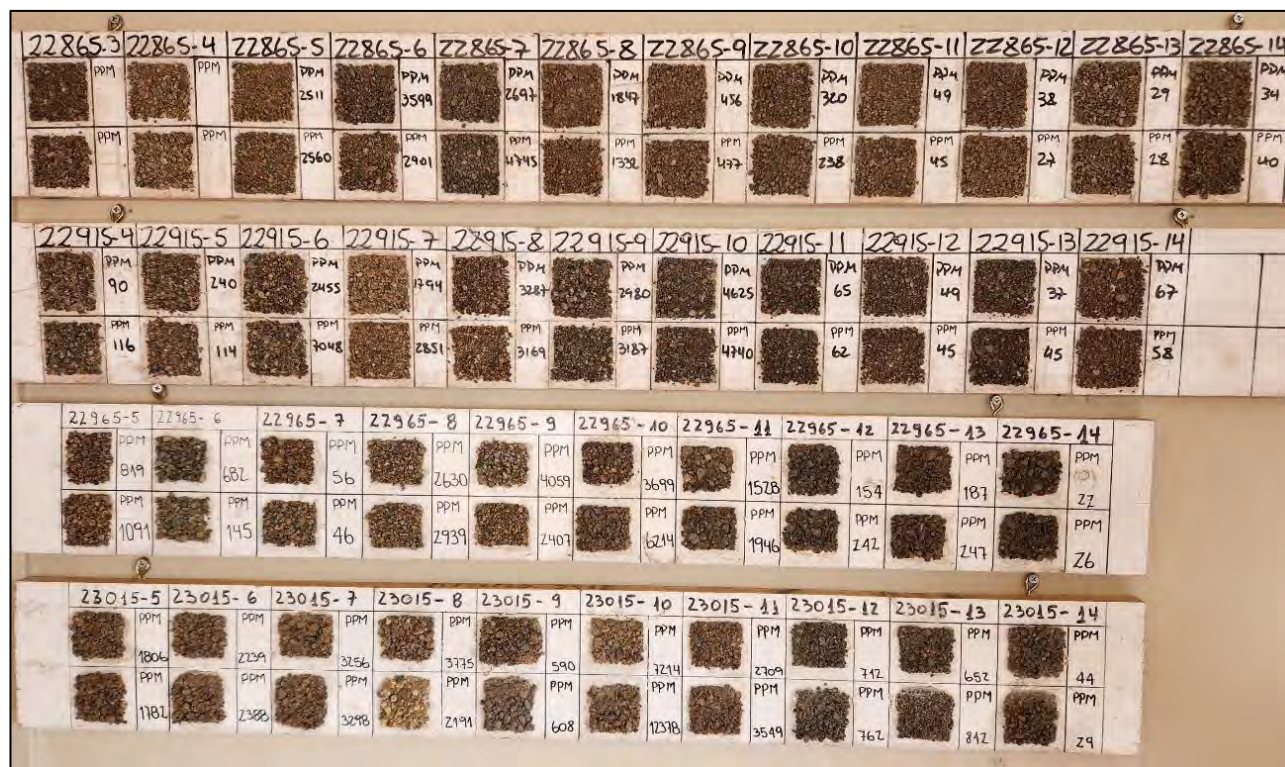
Figure 10-8. DTH coarse fraction samples with copper grades (ppm) hung on the wall of the field office for quick comparison between holes (Caracle Creek, 2024).
