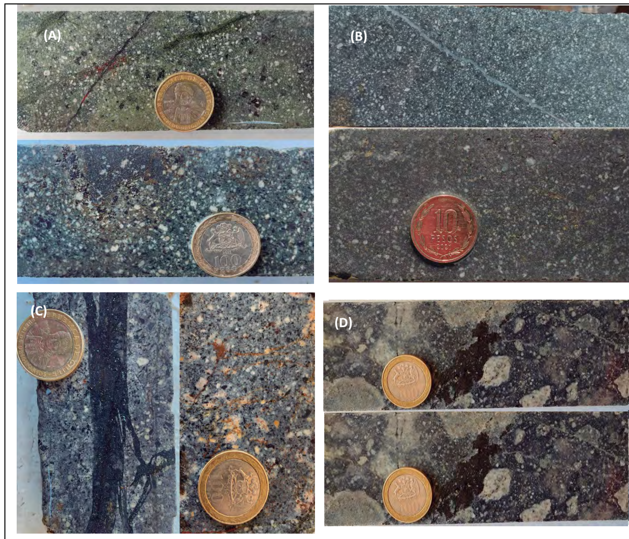
Figure 7-4. (A) Coarse-grained andesite (AND-G); (B) Fine-grained andesite (AND-F); (C) Andesite Porphyry (AND-P); (D) Volcanoclastic Breccia (BV) (Ptolemy Technical Services, 2024).
