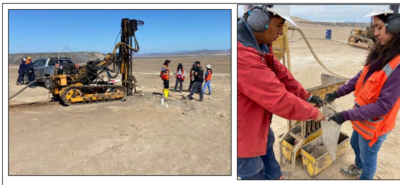
Figure 10-7. DTH air core grid-based drilling around diamond drill hole BRT-DDH-003. LEFT: Track-mounted air core drill rig set up. RIGHT: Riffle-splitting the sample after it has gone through a cyclone (Ptolemy Technical Services, 2024).
